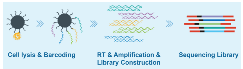
Figure 6: Single cells and barcoding beads are partitioned into the microwells (the chip can be visualized under the microscope). After cell lysis, the beads capture the RNA transcripts and render them with a unique cell barcode, as well as a unique molecular identifier (UMI). Following subsequent amplification and library construction steps, a single cell sequencing library that represents targeted analytes (mRNA, genetic variant, and more) can be sequenced to obtain complex genetic information from tens of thousands of cells, at single cell resolution.
